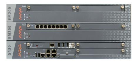
20 or 80 channel. The maximum capacity is 105 G.711/G.726 or 100 G.729 channels.
